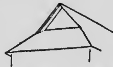
Combined Hip and Gable Roof.
