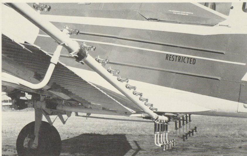
A Cessna Agwagon "B" is shown being loaded with insecticide. On the right, a view of the spray nozzles mounted along the wing trailing edge.
