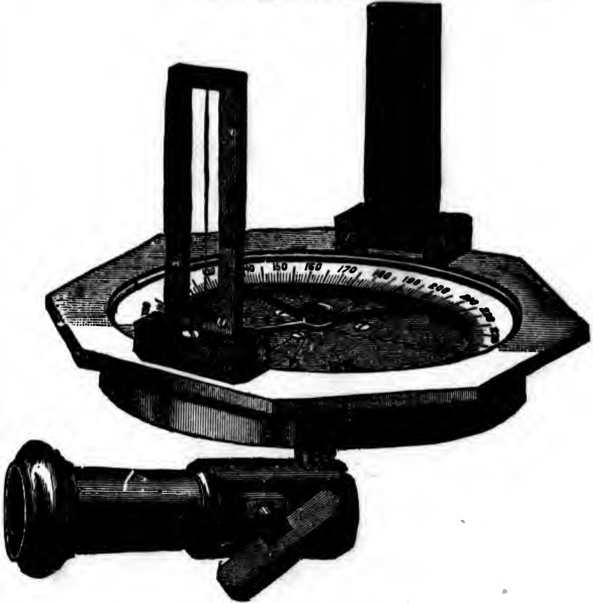
A COMPASS FOR SURVEYING LAND.
