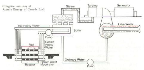
This simplified diagram shows how electricity is generated by the Candu natural uranium reactor. The natural uranium fuel in the reactor heats the heavy water, which in turn heats the ordinary water. The steam from the turbine, which drives the generator, produces the electric power. used — eliminates the expensive process for enriching uranium used in light water, and gas-cooled reactors.
