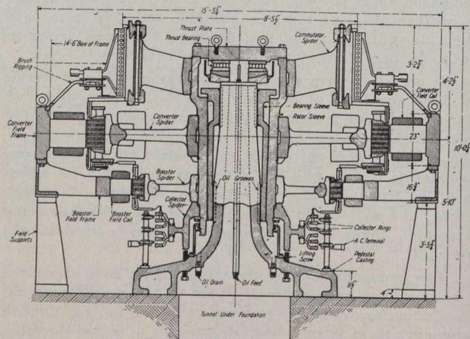
Fig. 2. Sectional View of 3000 kw. Vertical Converter.
