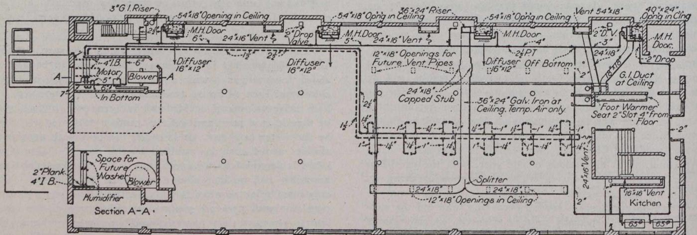
Basement Plan, Fan Heater Unit and Arrangement for Doubling the Capacity and the Steam and Air Distribution, Particularly for Second Floor.
