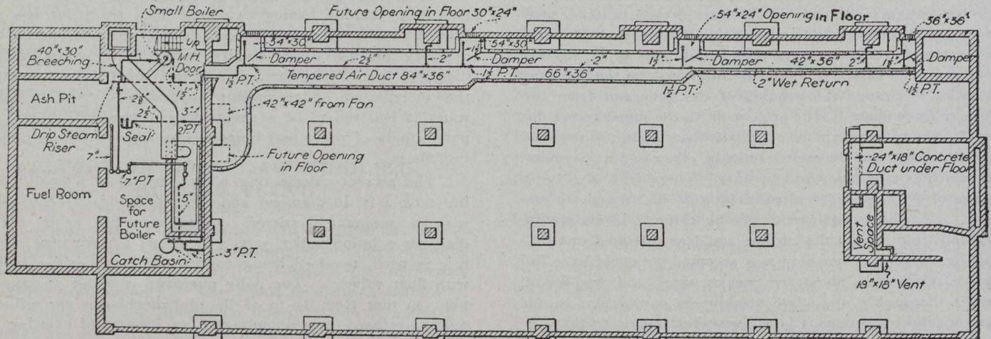
Basement Plan, Showing Tempered Air Duct Supplied by Fan on First Floor and Leading to Flues Containing Heating Surface.
