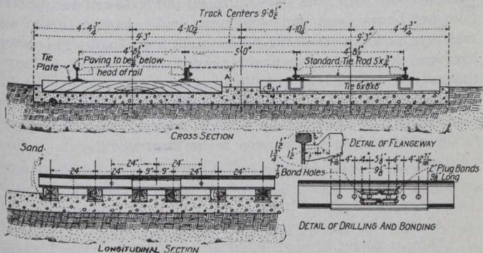
Fig. 1.—Standard Track Construction of British Columbia Electric Railway, Vancouver, B.C.
