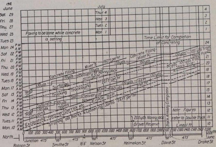
Fig. 2.—Progress Chart of Track Reconstruction Work.
