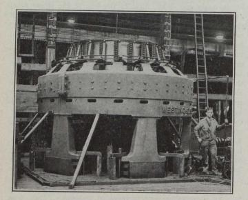
Fig. 1. 3000 kw., Vertical, Synchronous Booster, Commutating-Pole, Rotary Converter on Test,
