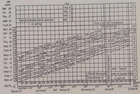
Fig. 2.-Progress Chart of Track Reconstruction Work.
