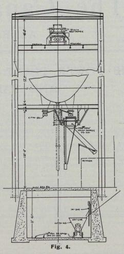
the storage pile by means of an orange peel bucket operated from a steam locomotive crane and loaded into a bottomdumping car. The locomotive crane is then used to shunt this car to a track hopper, into which the car is discharged. Under the track hopper is arranged a crusher and feeding-
