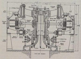
Fig. 2. Sectional View of 3000 kw. Vertical Converter.
