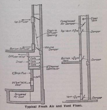
the room at the floor, but when cooling or merely ventilating, the exhaust air leaves the room at the ceiling. To this end, each supply flue and cach vent flue has two openings, with adjustable dampers in each.
