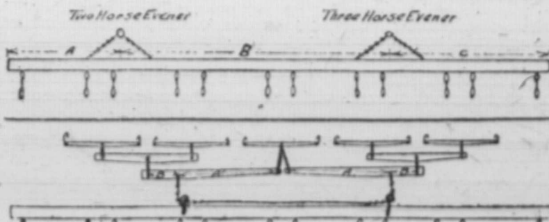
The upper half of this illustration shows how the horses might be hitched. The comparative lengths of the parts A, B, and C, are 2, 3, and 5, respectively. The lower half is a chain and pulley hitch easily arranged. The pulleys are at equal distance from the ends and the distance "A," i.e., from where the clevis holding the chain is attached to the centre of the draft which is at the centre of the middle whiffle-tree is four times the length of B. This illustrates the method mentioned in the accompanying letter.
