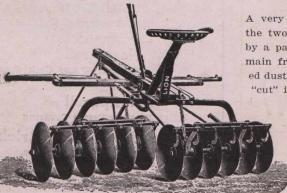
A very popular type. Staunchly built, the two disc sections are held in place by a particularly strong and rigid steel main frame, and run on highly polished dust proof bearings. The angle of the "cut" is controlled by one handy lever.
