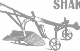
Natural temper steel blade. Weed Fender and gauge wheel. The Shaker Digger has a perfectly flat blade and will not cut the potatoes. The back grating shakes the earth clear and leaves the potatoes clean and on top of the ground.
