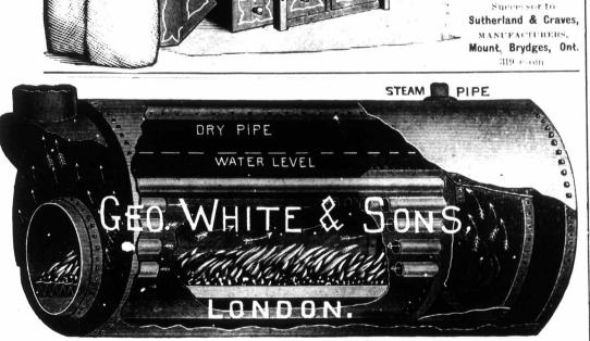
Whites' Wood and Straw-Burning Boiler. Special Internal Arrangements for Burning Straw.
