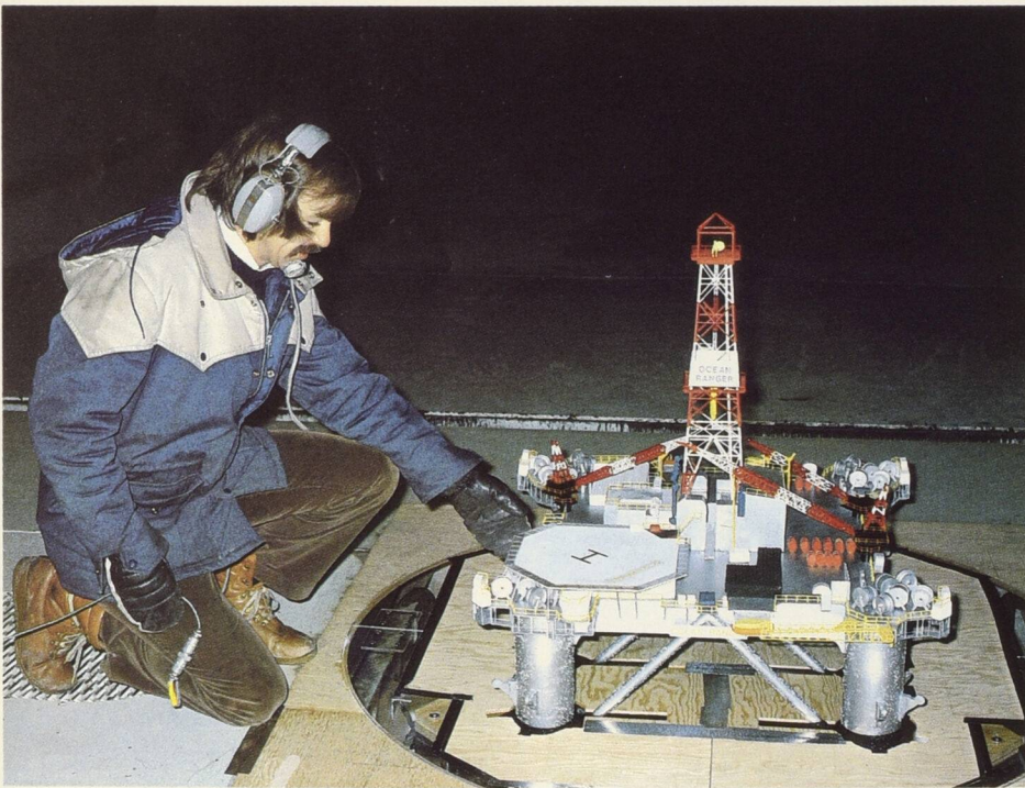
Bjarni Tryggvason of NRC's National Aeronautical Establishment prepares an oil rig model for wind tunnel tests. The wind dynamics data will be transferred to the Hydraulics Laboratory computer for use in conjunction with wave tests in the deep water tank.
