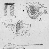
1. Empty Canister. 2 and 3. Canister Struck by Bullet After Being Filled with Water. 4. A Mauser Bullet After Striking.
