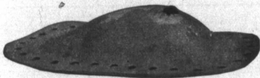
Bagged Plate, Caused by Scale.
