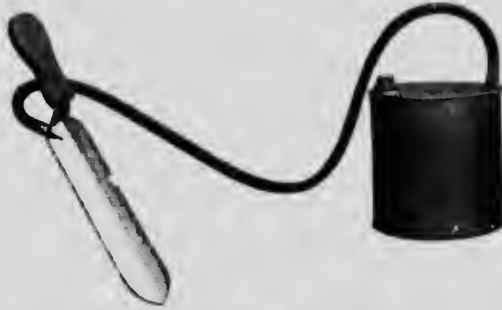
Fig. 19.—Steam heated uncapping knife with boiler.
