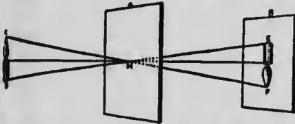
straight lines. Therefore, a ray of light from C must travel through the lens or hole H in the direction CF; and a ray from D must pass through H in the direction DE. If we hold a screen at B the image is caught in the position EF, upside down. For the same reason you always put the slides in a magic lantern upside down. Can you explain that to your own satisfaction?
