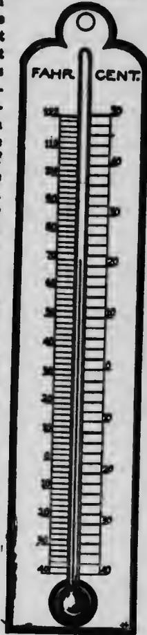
THE THERMOMETER Showing both Fahrenheit and Centigrade scales
