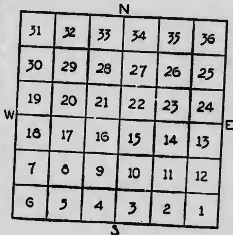
Each section is divided into quarter sections of 160 acres, and these quarter sections may be sub-divided into quarters. The numbering of the sub-divisions follows the same order as the numbering of the sections in the township, as shown by the diagram:
