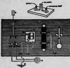
R, aerial; Q, binding post to aerial; C C' points to switch; H, busser; I, electro magnet; J, key or sounder; G, detector; A, armature of busser; N, binding post, connect to ground; P, binding post, connect to battery.
