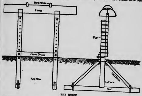
which should be made of two pieces of 2 x 4 x 9, cut rounding on one edge. Nail these handholds in place.
