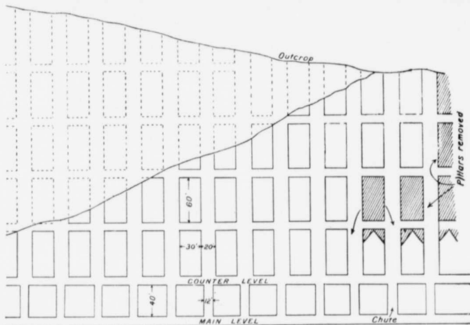
SKETCH SHOWING METHOD OF WORKING, DAVENPORT MINE
