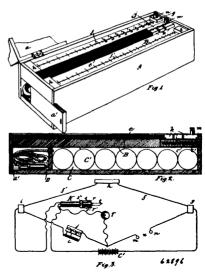
minals, insulated from each other, a metallic bar and two wires stretched between the respective blocks and the bar, said wires forming in series one side of the bridge circuit, a movable toucher and an indicating instrument in circuit therewith, substantially as described. 4th. In a Wheatstone bridge, the combination with the circuits thereof, of a bridge circuit closer and a battery circuit closer, combined into a single movable device, substantially as described.
