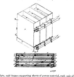
partitions being secured together to form closed compartments for the depolarizing agent, and spaces between each pair of said partitions for the exciting fluid, and positive electrodes in said spaces, substantially as described.
