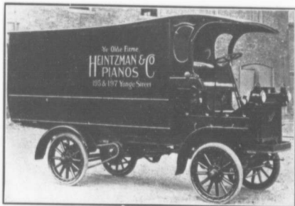
GRAMM 1 TON PIANO TRUCK with panel body 11 ft. long inside
