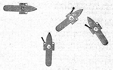
If A sees a White Mast-head Light above the Red Light, A knows that the vessel is a steam-vessel, and is either approaching her in the same direction, as B, or is crossing to port in some direction, as D D D.
