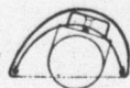
Fig. 2.—Show Case Reflector, 2 in. wide by 2 1/2 in. deep. Type used in Lipman Wolfe & Co., Inc., store.
