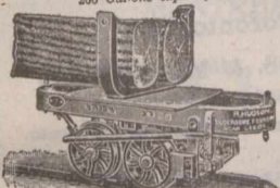
60—Bogie Wagon, with Swivel Fork for carrying Long Balcks
