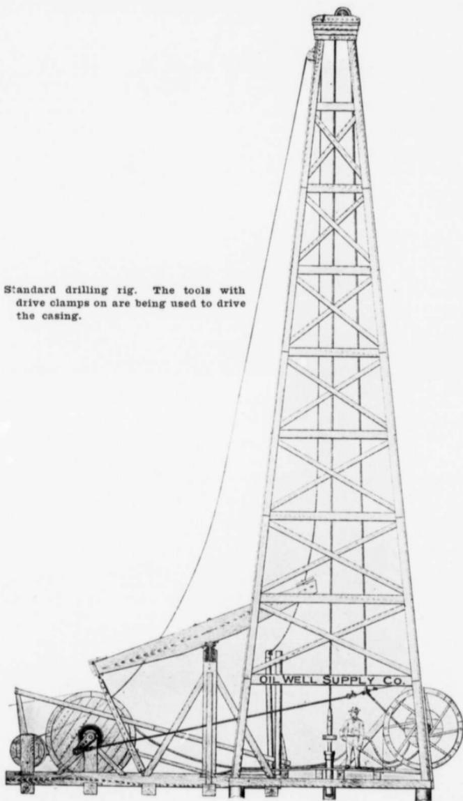
more easily shipped. In Australia, where white ants eat all articles of wood, steel is necessary. In Chili and Peru, on account of the excessive dryness in the rainless tracts, steel derricks are used. However, it is usually a question of taste upon the part of the manager of the properties as to whether wood or steel derricks are used.
