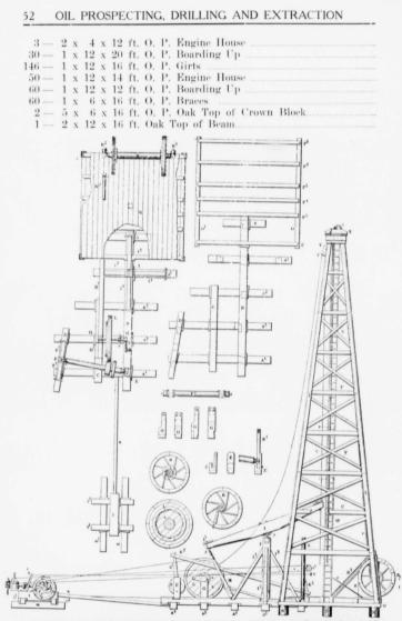
A derrick for standard drilling rig without calf wheel. The plan for ficor timbers is also shown. The floor construction is shown with location of bull wheel, belt wheel and sand reel. The construction of bull wheels and belt wheel is also shown.
