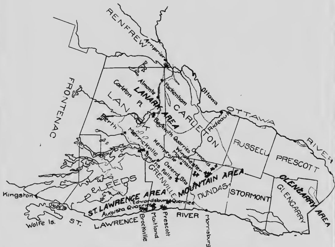
Fig. 13. Sketch map of part of Eastern Ontario showing the areas of the Beekmantown formation and the chief quarries.
