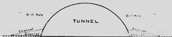
FIG. 7. Method of extending a tunnel laterally.
