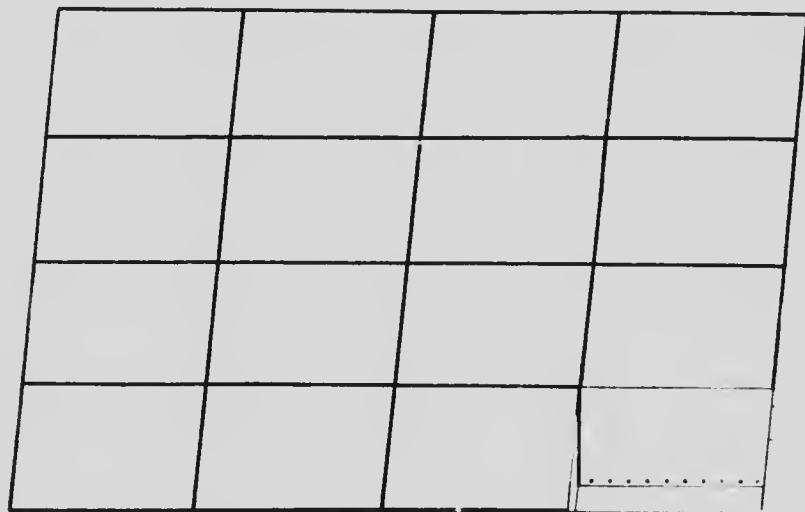
FIG. 5. Showing the floor of a quarry cut into rectangular blocks, the key block removed, and holes bored for raising the next block.
