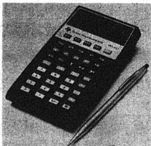
\*Performs all classical slide rule functions - simple arithmetic, reciprocals, factorials, exponentiation, roots, trigonometric and logarithmic functions, all in free floating decimal point or in scientific notation.
