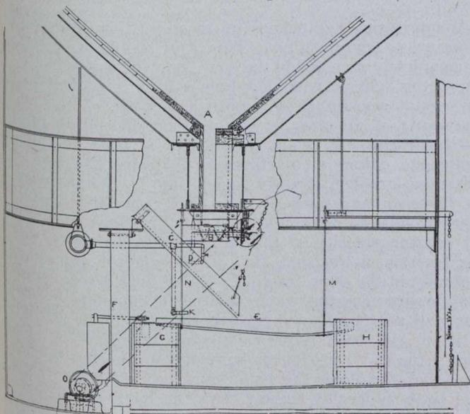
Fig. 1. GENERAL ARRANGEMENT OF CAMPBELL COAL WASHER.
