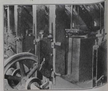
Rear view of Washing Tables, showing spray pipe, false bottom, sludge receiver, bumping post, cam and bumping device. Dominion Iron and Steel Co., Limited, Sydney, N.S.
