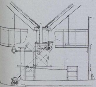
FIG. 1. GENERAL ARRANGEMENT OF CAMPBELL COAL WASHER.
