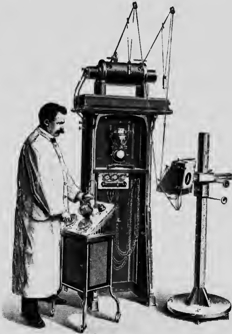
Fig. 310.—A COMPLETE MODERN X-RAY OUTFIT (except Couch), showing coil mounted up out of the way, interrupter beneath it, and all resistances and contacts mounted on a separate moveable stand. This apparatus (K. Schall & Son, London) uses continuous current from the main.
