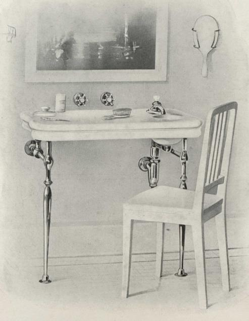
"ALEXANDRA WARE"—PLATE F. 093.—FIRST GRADE ENAMEL TOILET TABLE, WITH MANICURE BASIN, NICKLE-PLATED COMBINATION SUPPLY AND WASTE FITTINGS, WITH CHINA KNOB AND INDEX, 1 1-4 INCH ADJUSTABLE "P" TRAP ON WALL, NICKLE-PLATED BRASS FRAME AND LEGS. DIMENSIONS—LENGTH 33 INCHES; WIDTH, 18 INCHES; BASIN, 6 INCHES.
