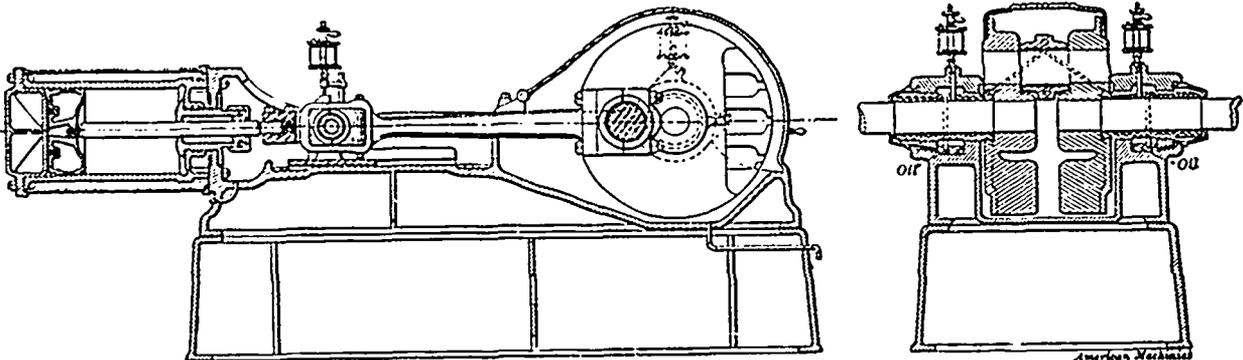
A small sight-feed oil cup, directly over the centre of the rocker arm, supplies oil through a tube to the outer end of the arm. The eccentric rod is hollow, being, in fact, a piece of hydraulic pipe, and through it the oil passes to the eccentric pin, any oil finally escaping being caught and held in the flanged fly-wheel.
