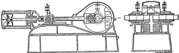
A small sight-feed oil cup, directly over the centre of the rocker arm, supplies oil through a tube to the outer end of the arm. The eccentric rod is hollow, being, in fact, a piece of hydraulic pipe, and through it the oil passes to the eccentric pin, any oil finally escaping being caught and held in the flanged flywheel.
