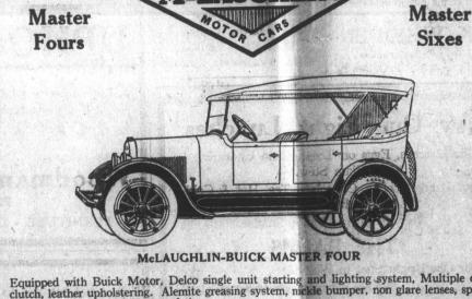
Equipped with Buick Motor, Delco single unit starting and lighting system, Multiple disc clutch, leather upholstering. Alemite greasing system, nickle bumper, non glare lenses, spiral bevel driving gear and 31x4 cord tires.
