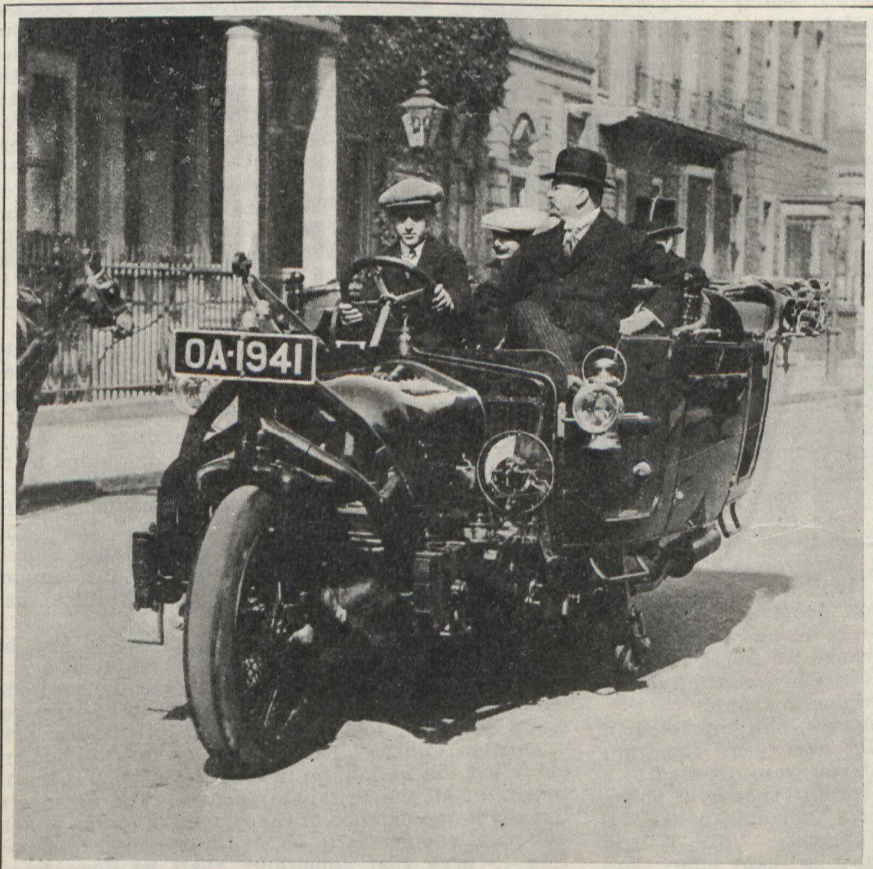
This six-seater motor runs on two wheels and is balanced by a gyroscope driven by electricity. The propelling power of the car is distinct from the driving of the gyroscope. Total weight, three tons. The photograph shows the car on its trial run in London with its Russian inventor sitting in front.
