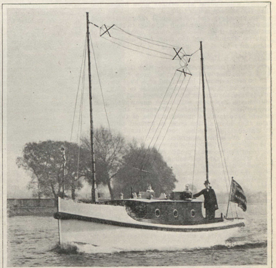
The new ocean monster, the Aquitania, will be equipped with two motor boats, thirty feet in length, and fitted with wireless apparatus with a range of about one hundred and fifty miles. People afloat in such a boat would be able to keep in constant touch with neighbouring steamers in cases of emergency.
