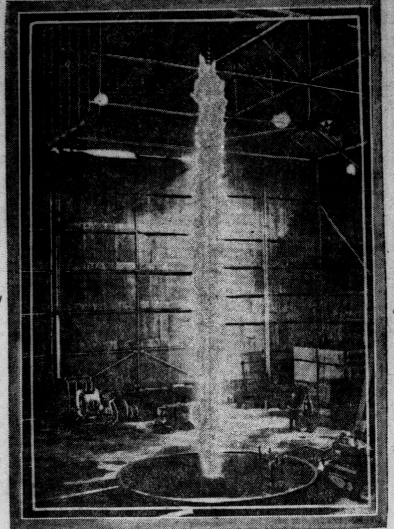
Making one million volts of electricity play tricks has recently been accomplished at an American laboratory. Photograph shows a forty-two-foot arc, said to be the largest controlled arc ever made
