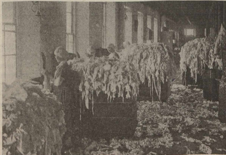
Huge boxes of rags are taken from the dusters to the sorting tables, where they are cut and freed from buttons and other substances not desired in a paper mill.
