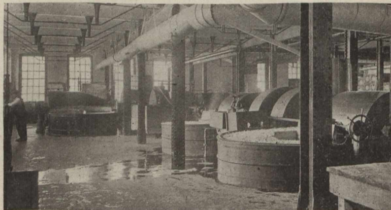
Beating is one of the most important operations. In this room we see the tubs with the stock circulating. In the rear beater on the left can be seen the revolving dipper that was spoken of in describing a washing engine. The beater in the foreground shows one end of the tub and the end of the midfeather. The hand-wheel turns a bar that extends across the beater and operates the lifting device which determines the position of the roll. The roll is protected and the stock is prevented from splashing out by the hood just behind the hand wheel. A box containing a filter cloth for straining the water to be used in the beater is shown just back of the tub.
