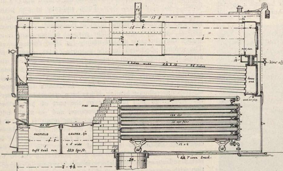
Fig. 1. The King Water Tube Boiler.
