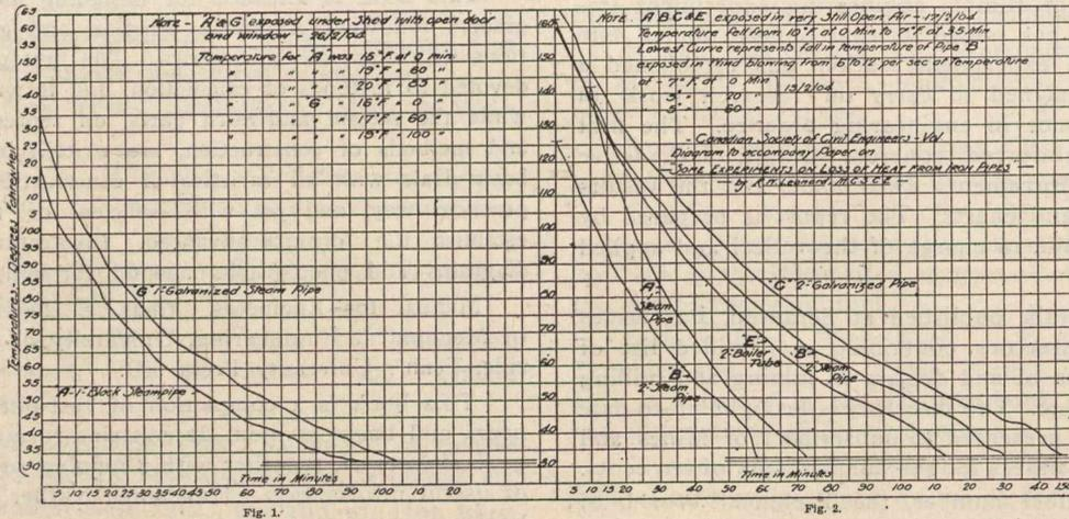
warmed loses its heat much more slowly when exposed to currents of cold air or water than when made hot. The practical application of this fact is that by forming ice racks of hollow tubes and connecting these tubes with a heating system, a remedy is provided for troubles from frazil ice. This remedy is especially applicable where there is a high head of water.
