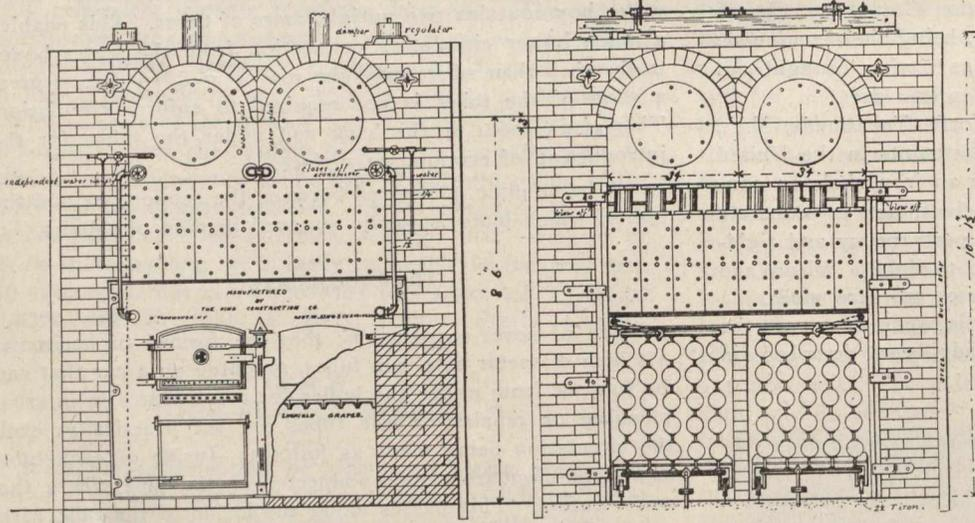
Fig. 2. Front View. Twin Setting. Back view door removed.
