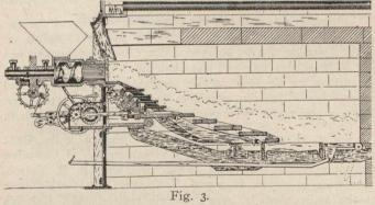
Section of King Automatic Stoker showing also bottom row of Boiler Tubes.
