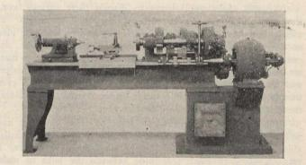
Electrically Driven Lathe-Back View.
