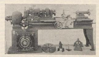
Electrically Driven Lathe-Front View.
