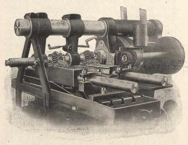
$4\frac{1}{2}$  in. in the rough, and the cut is  $\frac{1}{4}$  in. deep, added to which are the grooves, one of which is  $\frac{7}{8}$  in. deep and 21-32 in. wide. The cutters are made of Novo steel, and are 4 in. and  $\frac{53}{4}$  in. in diameter. The work is fed through the machine 15-16 in. per minute, and the finished surfaces are smooth and accurate.
