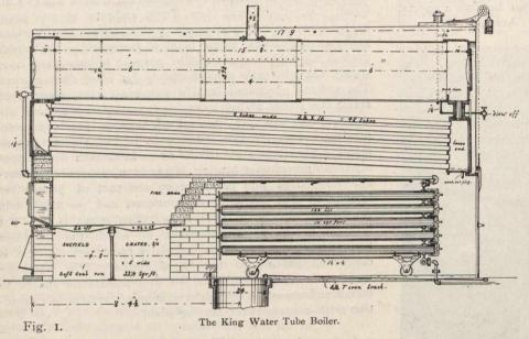
fire doors, from which will extend loops of tubes which will support the fire crown. Removable covers on the water front will enable the inside of tubes to be cleaned of scale. Water will circulate through the tubes—by this arrangement a fire crown of any width can be supported.
