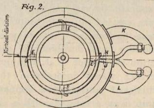
vided in the annular trough, forming the compartments H and J, each of which measures at the circumference 1 per cent. of the total circumference of the annular space. It is evident, therefore, that these radial compartments will each withdraw 1 per cent. of the total amount of water passing from the turbine, no matter what the quantity flowing may be.
