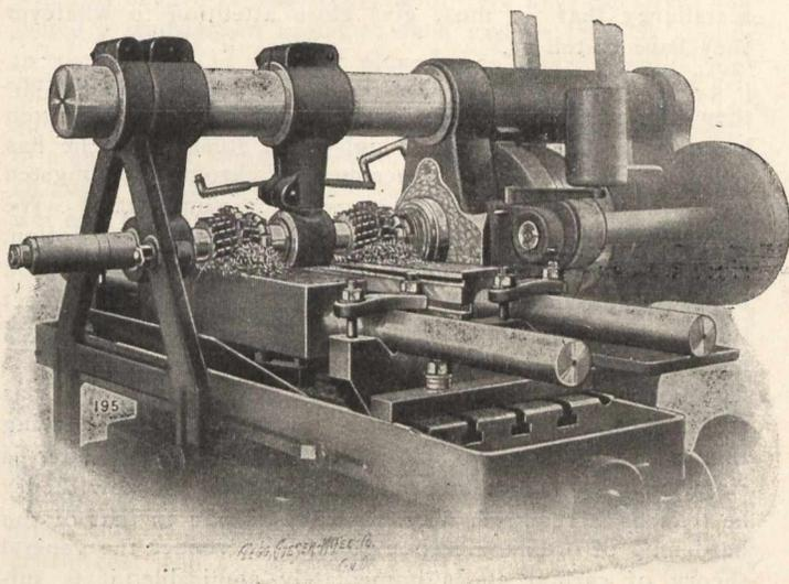
4½ in. in the rough, and the cut is ¼ in. deep, added to which are the grooves, one of which is ⅞ in. deep and 21-32 in. wide. The cutters are made of Novo steel, and are 4 in. and 5¾ in. in diameter. The work is fed through the machine 15-16 in. per minute, and the finished surfaces are smooth and accurate.
