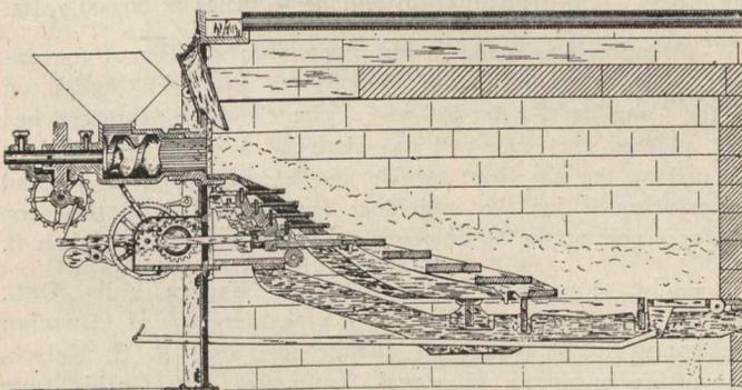
Section of King Automatic Stoker showing also bottom row of Boiler Tubes.
