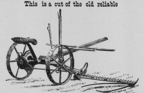
COSSITT BUCKEYE MOWER. improved for the season of 1893. The removal of the Leading wheel and the light Malleable inside shoe allow perfect freedom of tilt and with the improvement in the shifting gear constitute it the lightest draft
