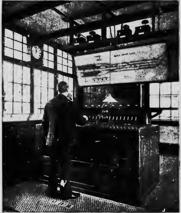
In a railway signal-box. Note the levers for working the signals, and the plan of the railway lines in front of the operator.
