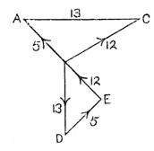
4. (b) Let t = tension in BA t' = tension in BC.  $\triangle$  BDE has its sides parallel to direction of forces t. t' and 65.
