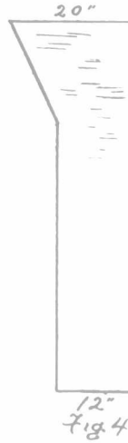
Fig. 4 Cross Section of Concrete Wall.
