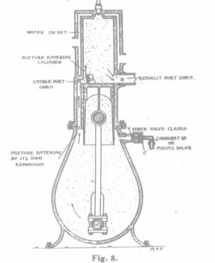
Compression stroke of four-cycle engine. Both valves closed. Up-stroke of two-cycle engine. Compression in the cylinder, mixture taken into base. Intake and exhaust ports closed. Two-cycle engine, with exhaust port and intake port both open. Mixture entering cylinder by expansion from base. Exhaust and intake occur together and almost instantaneously.
