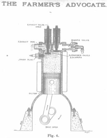
Intake stroke of four-cycle engine. Intake valve open. Piston moving down. Mixture being drawn in, The intake valve may be opened by a push rod or by suction. Exhaust stroke of four-cycle engine. Exhaust valve open. Piston moving up. Expanded gases being expelled. Exhaust valve opened by a push rod.
