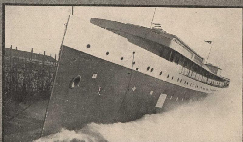
The Hamonic—1. Laying the Keel in June. 2. As she appeared in September when the third deck was reached. 3. Ready for Launching, with part of the Aerial Railway taken down for this purpose. 4. As she slid into the water of the Dry-Dock.
