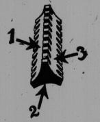
The Sunshine Furnace grates have three lives-that is, they have three different surfaces to be exposed to the heat and wear. The surfaces are alternated at will, with little effort, so that there is three times as much wear in Sunshine Grates as there is in the ordinary one-surface grate.
