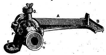
The Disks are tempered and have very hard cutting edges, not liable to break or to wear easily.
