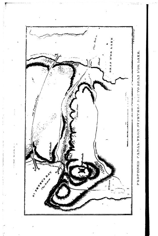
By adopting this line A. B. the entrance Lock in St. Peter's Bay must be strongly protected by Piers, and a Breakwater of Masonry; this point being exposed to the action of the sea, during all gales from the south and south west. Here the beach is composed of sand and the water shallow.
