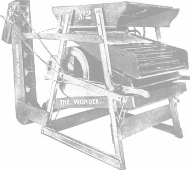
The gang of **FIVE ZINC SCREENS** used in the upper shoe for wheat (the top sieve covered with oil cloth) makes it practically impossible for the oats to pass through with the wheat.
